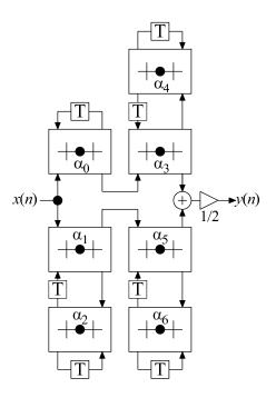
• Number the nodes and operations and create the signal flow graph. The inputs and outputs of the symmetric two-port adaptor are related and numbered as shown below. Note that the position of the adaptor coefficient,  $\alpha_0$ , denotes which input to be subtracted.
