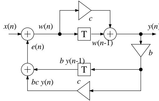
Apply the  $z$ -transform to the difference equation to obtain the transfer function
