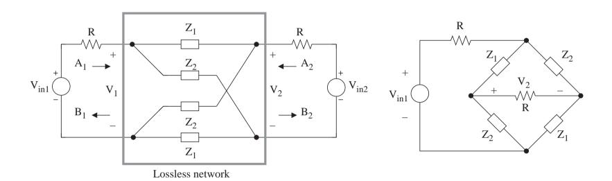
Note that the lattice structure is in fact a bridged structure. Thus, the lattice structure is extremely sensitive to element errors in the stopband.
