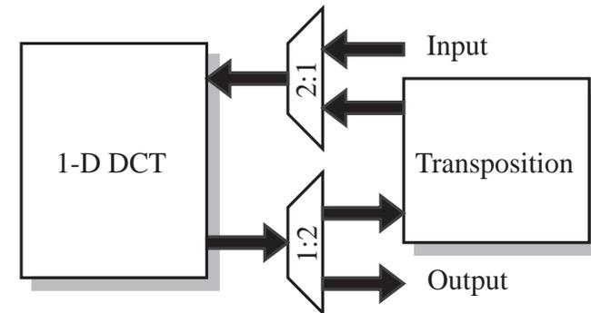
In the second phase, the columns in the intermediate array are successively computed by the processing element.
