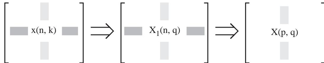
$2N$  one-dimensional DCTs and one matrix transposition of the intermediate data array are needed. A computation, based on one-dimensional DCTs, requires  $2N^3$  multiplications per block.
