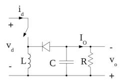
5. A 3V negative output voltage (V<sub>0</sub>) is generated using the buck-boost converter below. The input voltage V<sub>d</sub> is 12V. The converter is running in continuous conduction mode. Assume C is large.  $L = 38.4 \mu H$ , T<sub>s</sub> = 20 µs.
