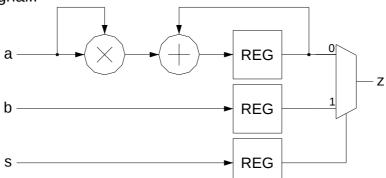
• If the critical path is defined by the multiplier and the adder, how can we now reduce and, thus, increase the clock frequency?
