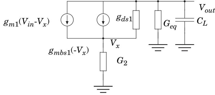
**Figure 2.2** The small-signal model of the amplifier.
