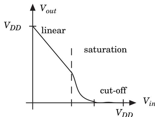
**Figure 1.1** The output voltage as a function of the input voltage.
