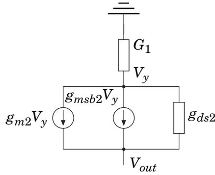
**Figure 2.1** The small-signal model of the PMOS part of the amplifier.
