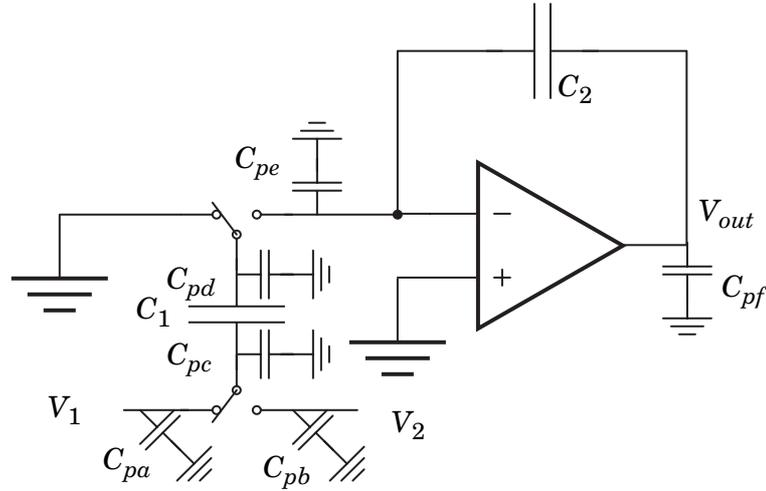
**Figure 4.1** SC circuit with capacitive parasitics.
