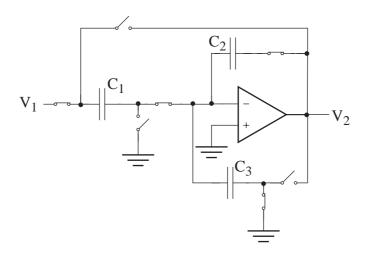
Figure 4.1 A switched capacitor circuit
