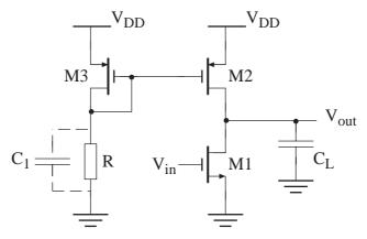
Figure 3.2 A noisy common source gain stage
