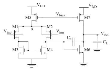
Figure 2.1 Operational transconductance amplifier
