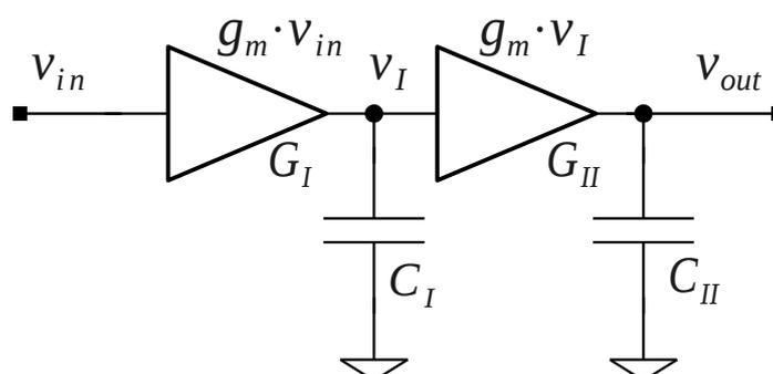
Figure 3.1: A two-stage amplifier.
