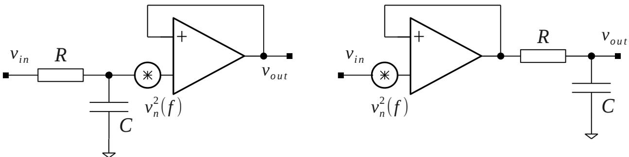
Figure 2.1: A buffer and some passive circuit.
