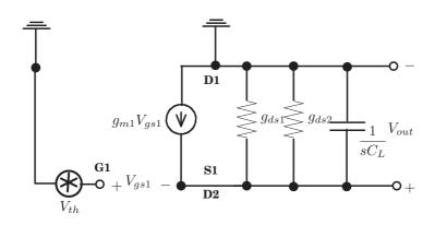
Figure 4: Small signal equivalent circuit.
