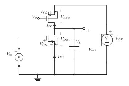
Figure 1: Inverter. Large signal analysis.
