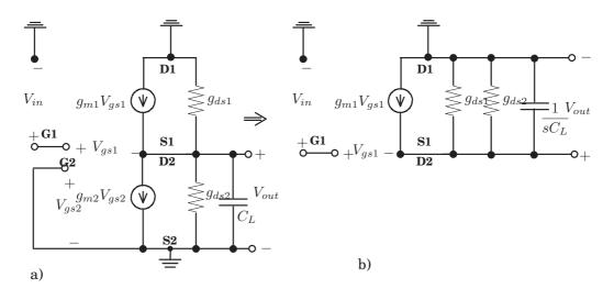
Figure 3: Small signal equivalent circuit.
