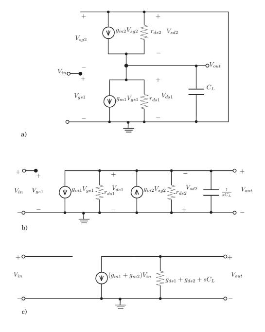
Figure 2: Complete small signal equivalent.
