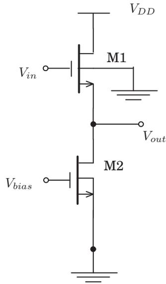
**Figure 1:** Simple gain-stage.
