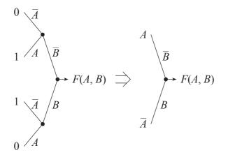
Replace the branches with NMOSFETs and add an inverter to the output. The complementary output can e.g. be realized by inverting the inputs to the tree like resulting in the circuit shown to the left below.
