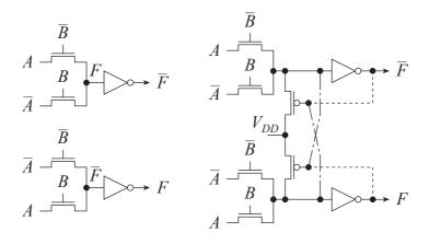
b) Add keepers to the nodes with reduced swing before the inverters as shown above to the right. The gates of the keepers can be connected in two ways:
