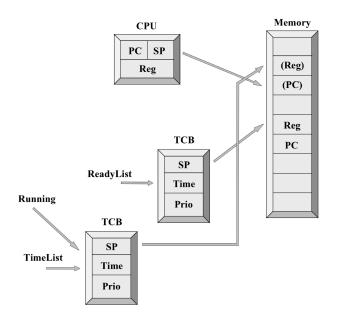
Figure 2: Two tasks, where the task marked Running is executing. The task control block of the executing task has been moved from ReadyList to TimeList, as a preparation for a task switch.
