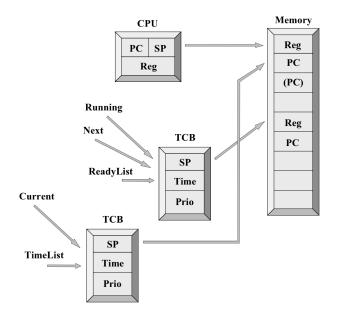
Figure 3: Two tasks, where the task marked Current is executing. Context for the running task has been saved, on the running task's stack.
