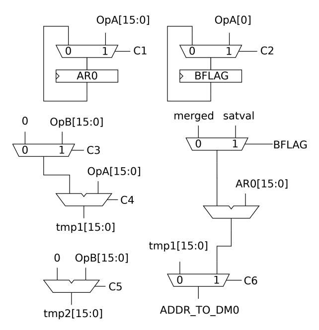
Assumptions made in this solution: There are two inputs to the AGU from the general purpose register file: OpA and OpB, each 16 bits wide. One of these inputs (OpB) can carry an immediate as well.
