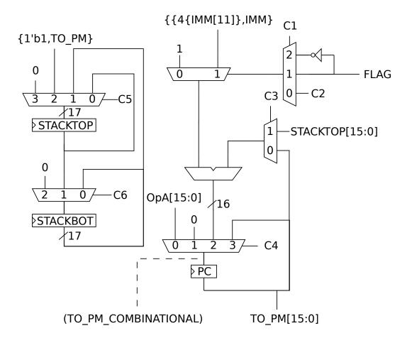
*Note:* In a real processor it may be a pretty good idea to take the output to the program memory from the TO\_PM\_COMBINATIONAL signal since the PM most likely has registers at the address inputs. (Either alternative is ok on the exam though.)
