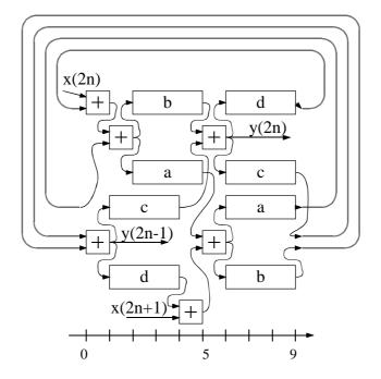
4. a) Name additions A1 to A3 from left in the figure. Draw an inclusion graph (connect nodes where the corresponding operations can share a resource). Find the minimum number of cliques (fully connected subgraphs). This can be difficult as there are a lot of edges in the graph. An alternative solution is to use an exclusion graph, where an edge defines that the connected operations can not share a resource.
