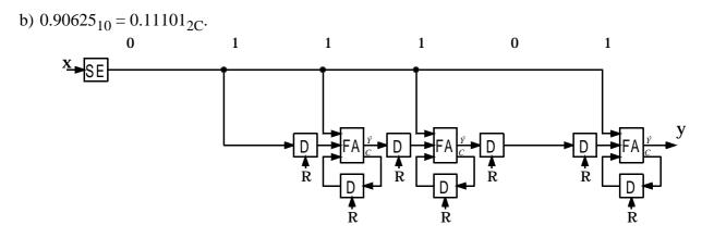
c)  $0.11101_{2C} = 1.00 \cdot 101_{CSDC}$ . Note that the initial 1 is not of weight -1 but of weight 1. (Compare with 2's complement where the sign bit has a weight of -1). The S control signal is setting the value of the flipflop to 1 at the start of the calculation. Another equally correct solution would be to use  $0.11101_{2C} = 1.000 \cdot 1 \cdot 1_{SDC}$ .
