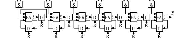
The structure is reset at the start of the calculation using the signal R. The block SE is extending the sign by copying the sign bit. It is also possible to replace the first step with a subtraction of x times a0. The feedback of the first bitslice would then be removed, and the carry flipflop should be set instead of reset at the start of the multiplication.
