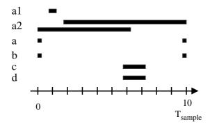
Note that there are variables that lives longer than a single sample period. Must therefore draw a lifetime diagram for two sample periods. Add a and b to the names to indicate first or second sample period.
