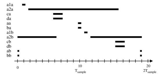
Allocate one memory cell and assign variables by traversing the list from beginning. Allocate cells until every variable in the list has been assigned to a memory cell.
