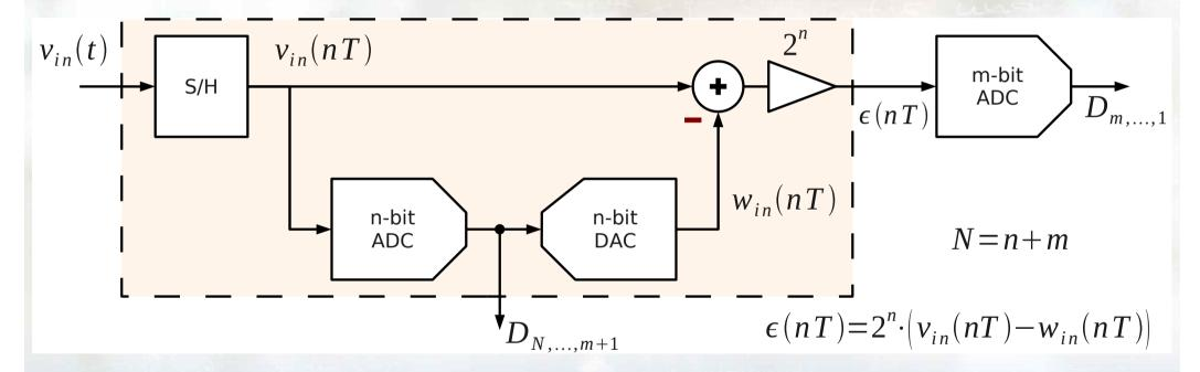
Another analog adder is required as well as a gain circuit, which limits the speed.
