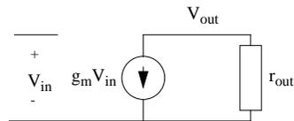
$$A_v = \frac{V_{out}}{V_{in}} = -g_m r_{out} = -g_m (r_{ds1} \parallel r_{ds2})$$
