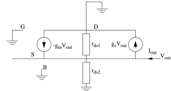
The output resistance is derived for zero input signal. Nodal equations:
