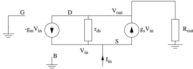
When using y- or z- parameters to derive the input impedance, either the output current or the output voltage should be set to zero. When analysing circuits where the input resistance depends on the load impedance (the CG stage is such a circuit) it is more convenient to include the load in the analysis and leaving the output open. This has been done in the above small signal model and gives the following nodal equations:
