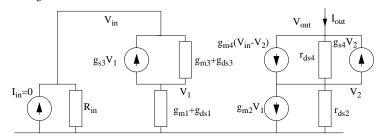
When calculating the output resistance, variations in the output voltage and the output current are considered. All constant voltages and current that are not affected by variations in output current or voltage are set to 0. This is the case for  $I_{in}$  and since no currents or voltages in the input circuit is affected by the output circuit we have  $V_1 = V_{in} = 0$ . The resulting nodal equations are thus
