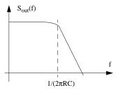
By using the noise bandwidth  $NBW = \frac{\pi}{2} f_{-3dB} = \frac{\omega_{-3dB}}{4}$  we have
