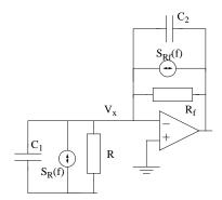
Ideal opamp =>  $V_x = 0$ . We have contributions from two noise sources. The transfer function from input current to output voltage is given by:
