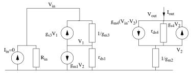
If we compare this circuit to the one in 3.13 we see that in this case transistor M1 has its gate connected to the output circuit. Thus we can **not** assume that  $V_{in}$  and  $V_1$  are 0. The input source is not affected by the output circuit and can be set to 0, i.e.  $I_{in} = 0$ . The resulting nodal equations are thus
