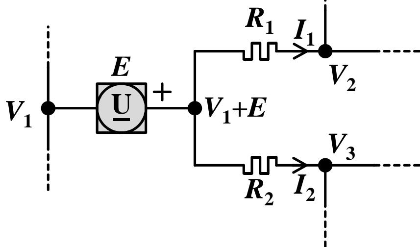
$$I_2 = \frac{V_1 + E - V_3}{R_2}$$
