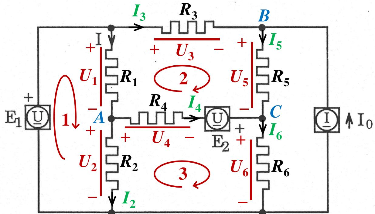
$$U_1 = R_1 I_1 \quad U_4 = R_4 I_4$$
