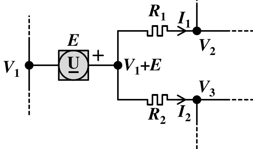
$$I_2 = \frac{V_1 + E - V_3}{R_2}$$
