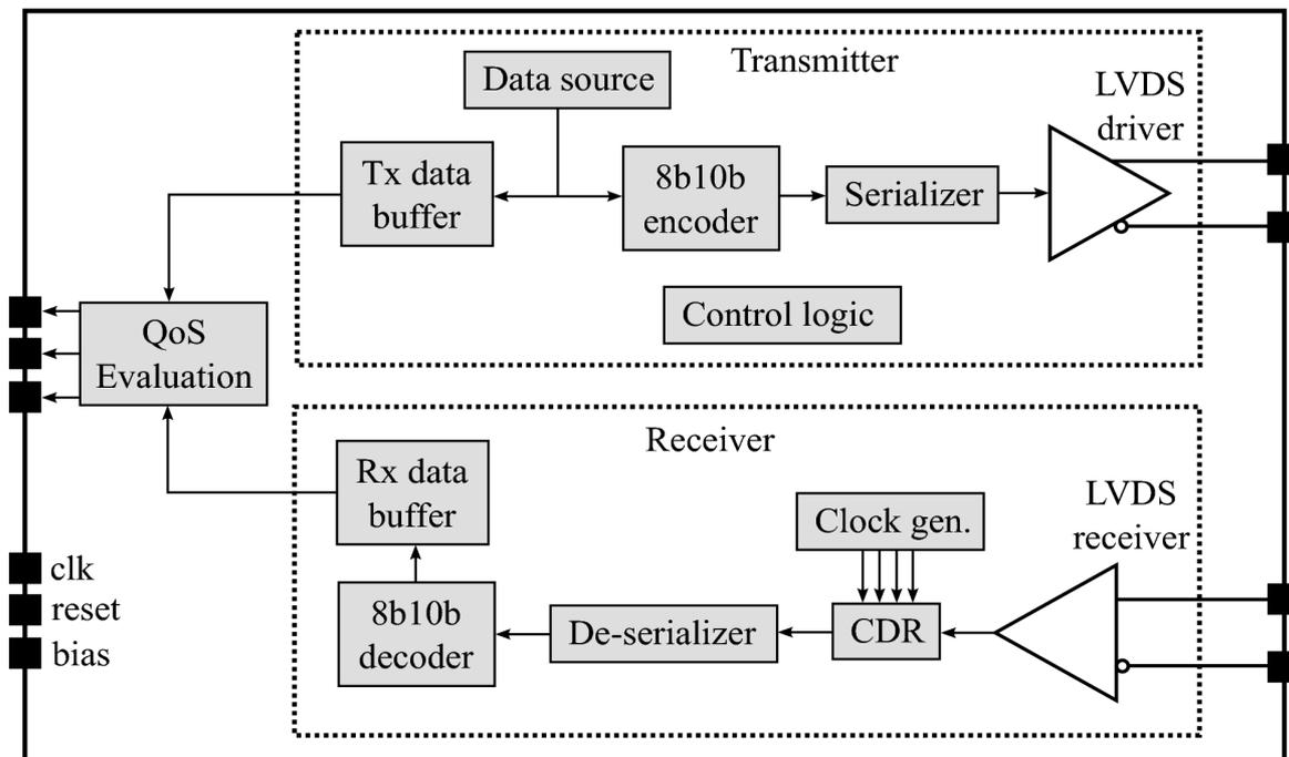
Figure 1: High speed serial link transceiver system overview.
