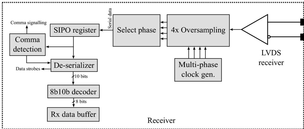
**Figure 2: Detailed receiver architecture.**
