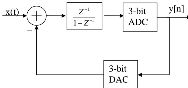
Figure 1: First-order Sigma-Delta modulator architecture.
