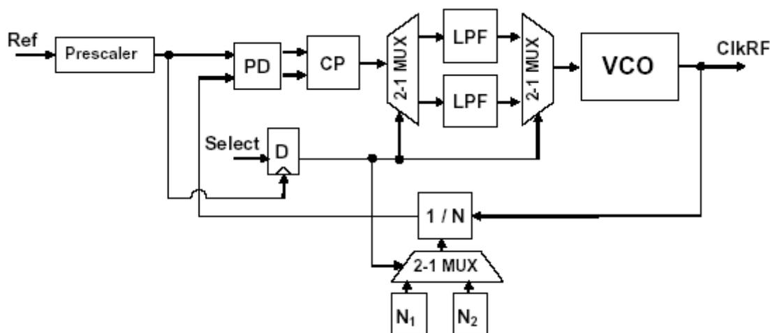
Figure 1: System Block diagram of PLL-based BFSK Modulator
