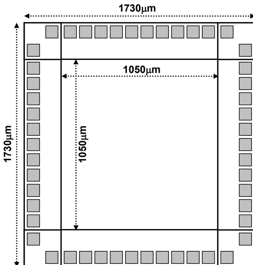
Figure 2: Schematic picture of a 3mm<sup>2</sup> chip with 40 generic pads four  $V_{DD}$  and four  $V_{SS}$  pads (total 48 pads), which will be shared between a number of projects.
