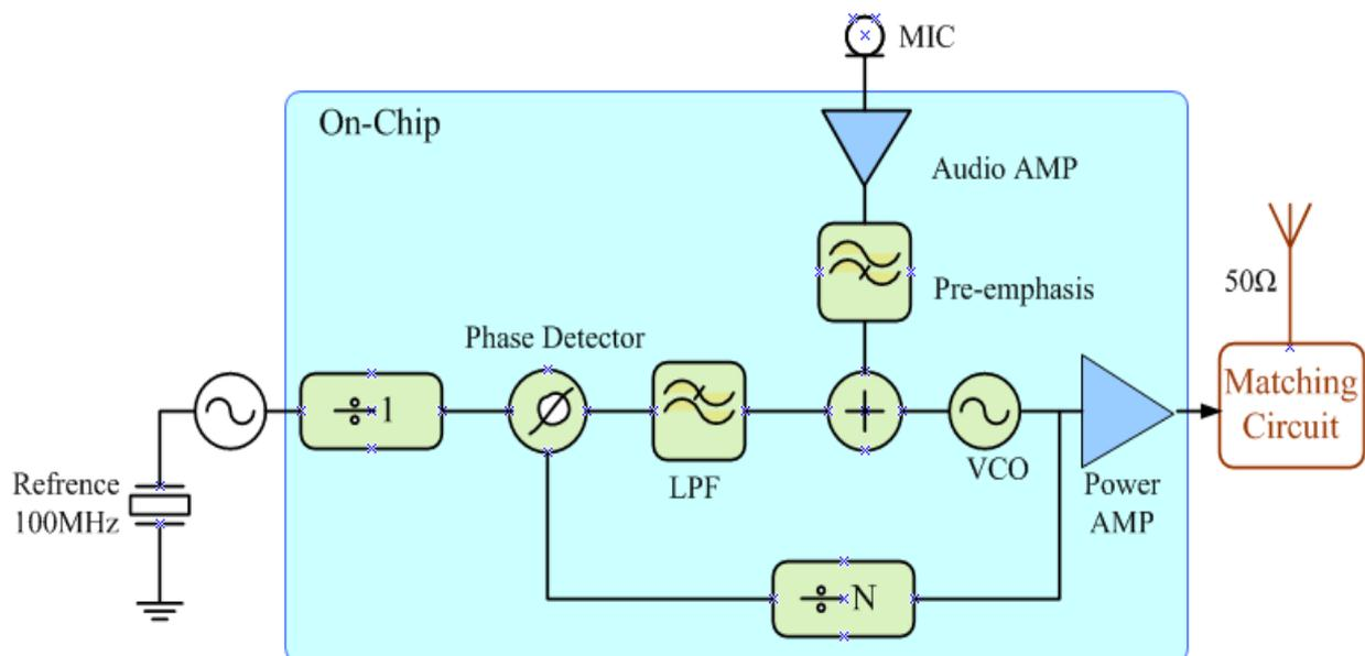
**Figure 1: System Block diagram of 100MHz, 10dBm direct VCO modulating FM radio Transmitter.**
