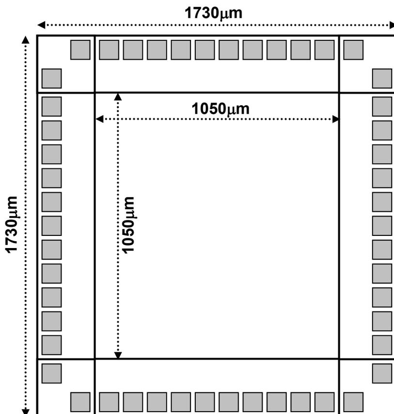
Figure 3: Schematic picture of a 3mm<sup>2</sup> chip with 40 generic pads four  $V_{DD}$  and four  $V_{SS}$  pads (total 48 pads), which will be shared between a number of projects.
