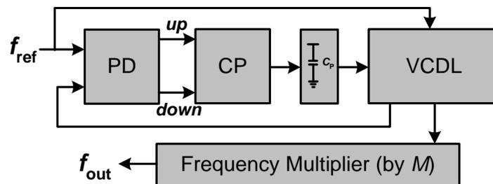
Figure 1: System Block diagram of DLL-based frequency multiplier.
