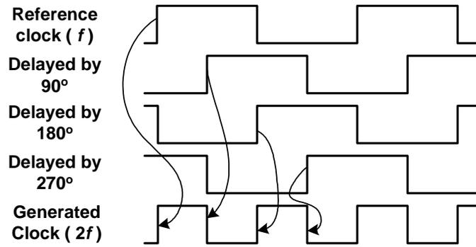
Figure 2: Example of timing for a frequency multiplier
