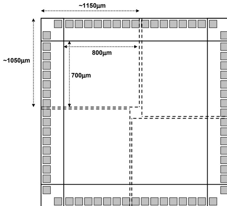
Figure 2: A 5mm<sup>2</sup> chip will be shared by 4 independent projects (4 teams). Each project will utilize a 700x800μm<sup>2</sup> area for core layout and 17 pads.
