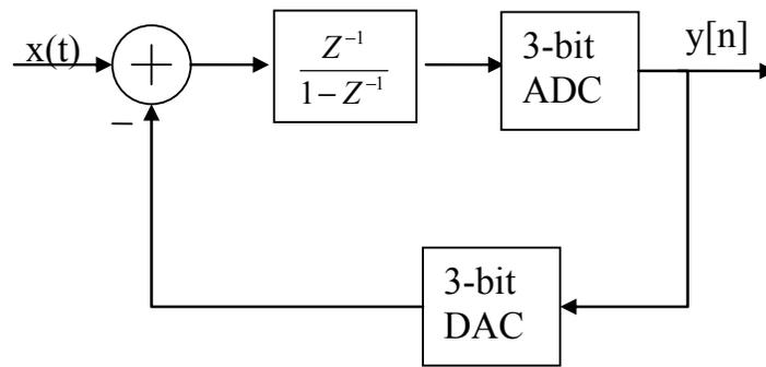
Figure 1: First-order Sigma-Delta modulator architecture.
