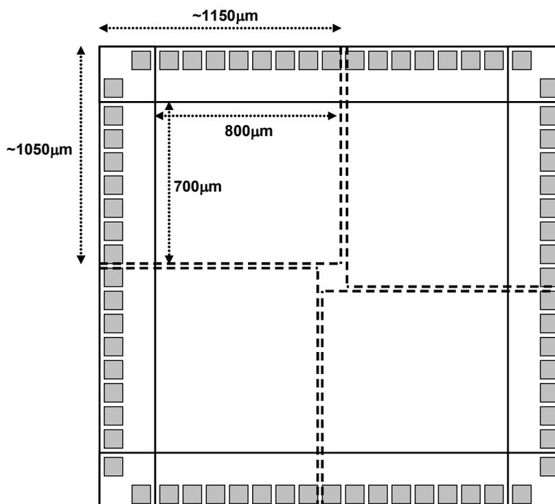
Figure 2: A 5mm<sup>2</sup> chip will be shared by 4 independent projects (4 teams). Each project will utilize a 700x800µm<sup>2</sup> area for core layout and 17 pads.
