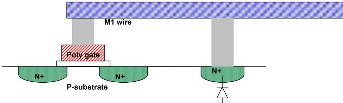
Long metal wire with reversed diode to substrate.
