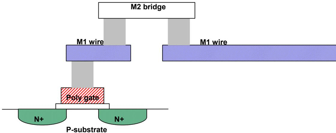
Long metal wire broken up by a bridge in higher or lower layers
