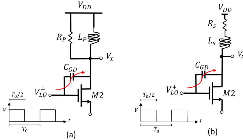
Fig. 2.2 (a) Single-ended with LO-IF feedthrough (b) transformation from parallel to series
