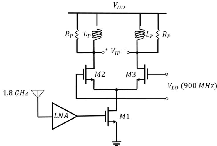
Fig. 2.1 Receiver front-end
