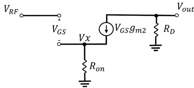
Fig. 3.2 Small-signal model with on-resistance  $R_{on}$
