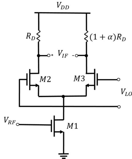
Fig. 1.1 Active mixer with load mismatch
