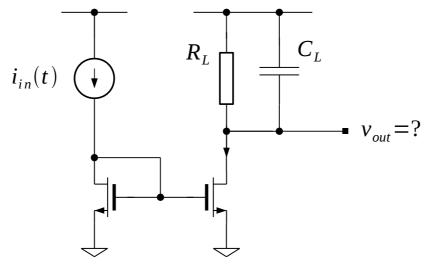
Figure 1.1: Current mirror with passive load.
