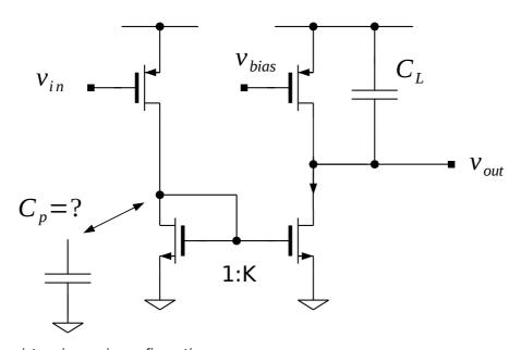
Figure 3.1: Transistors in a gain configuration.
