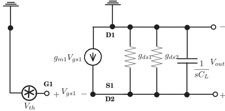
**Figure 4:** Small signal equivalent circuit.
