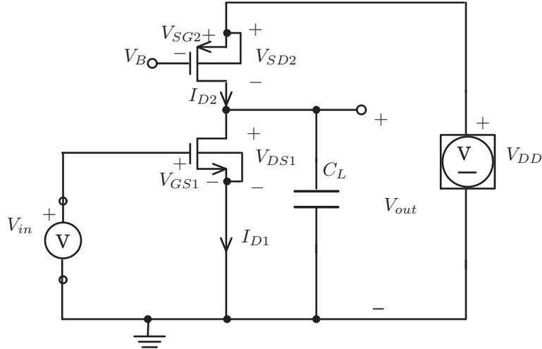
**Figure 1:** Inverter. Large signal analysis.
