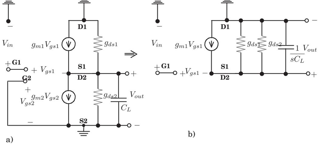
**Figure 3:** Small signal equivalent circuit.
