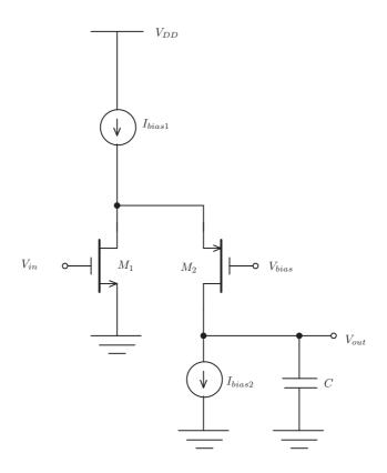
Figure 2: Folded cascode stage.
