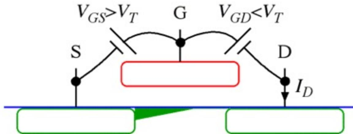
Saturation region:  $V_{GS} > V_T, V_{DS} > V_{GS} - V_T = V_{GT}$
