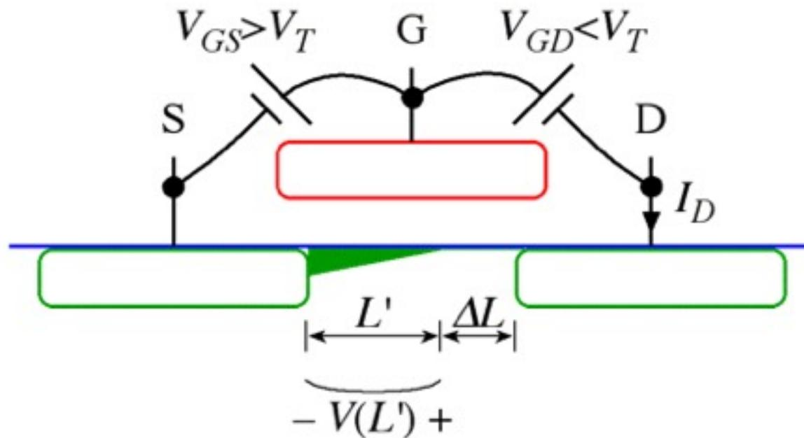
Channel is pinched off at  $L' \Rightarrow V(L') = V_{GS} - V_T = V_{GT}$
