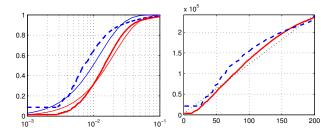
Figure 6. Left: Empirical CDFs and the approximating  $\mathcal{X}_3^2$  CDFs on a logarithmic scale. Solid curve is empirical distance CDF for the original image, dashed curve is distance CDF after Gaussian blur. Thin curves are approximating  $\mathcal{X}_3^2$  CDFs. Right: The resultant number of edges processed after each time step. Dotted straight line is desired curve.
