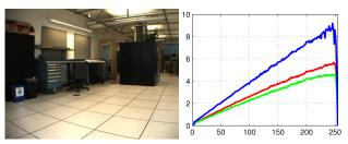
Figure 4. Image variance as function of intensity. Left: Mean image of 100 identical frames. Right: Variance from mean as function of intensity for the three colour bands.
