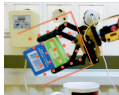
Visually controlled low-cost robot, holding an object that has been automatically detected and analyzed.
