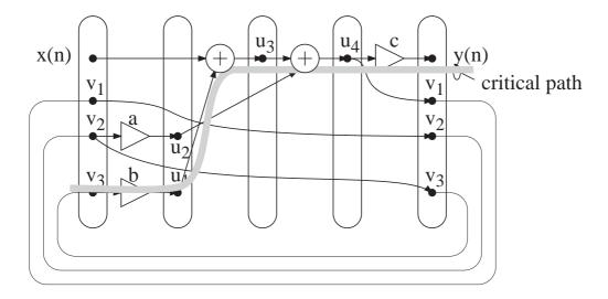
Since the critical loop is large than 1 sampling period, we have to schedule the operations in two sample periods. The scheduling with the maximal sample frequency is shown below.
