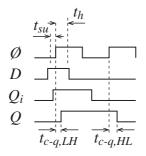
Setup time  $t_{su}$ : The time before the rising edge of the clock that the input data D must be valid.
