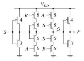
b) Aspect ratios are indicated directly by the transistors in the schematic above.
