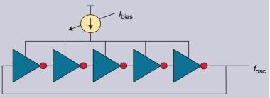
Current-Starved Ring Oscillator;  $f_{osc} = n/t_d$ ;  $t_d \sim 1/I_{bias}$
