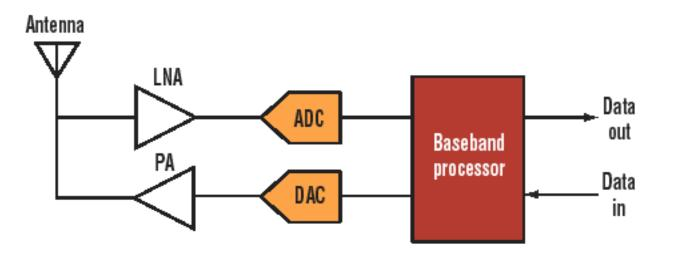
1. In the ideal software-defined radio, the antenna connects directly to the LNA and ADC, or the PA and DAC. The processor handles all radio functions, filtering, up/downconversion, modulation/demodulation, and digital baseband.
