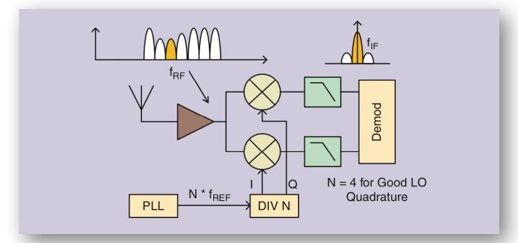
"Quadrature LO" => PLL at 2x or 4x RF frequency => high power consumption.
