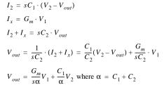
With this circuit we can perform an addition and an integration.
