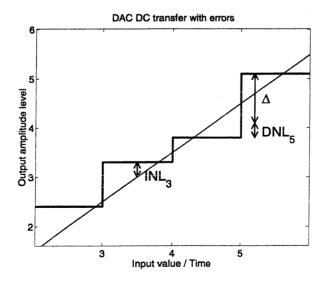
(<u>Monotonicity</u> of a DAC is when the output always increases for increasing input)
