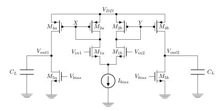
Figure 2: A fully differential amplifier.
