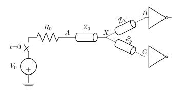
Figure 4: Transmission line circuit.
