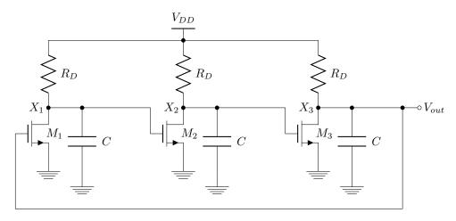
Figure 5: 3-stage ring oscillator
