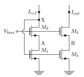
Figure 3: A low-voltage cascode current mirror.
