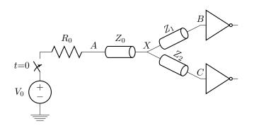
Figure 4: Transmission line circuit.
