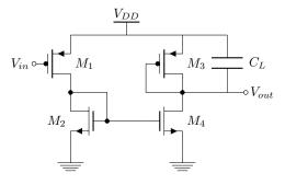
Figure 1: Schematic of a single-ended amplifier.
