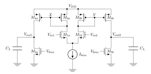
Figure 2: A fully differential amplifier.
