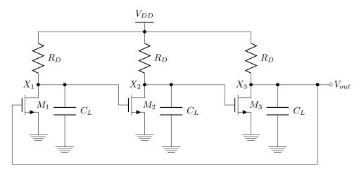
Figure 5: 3-stage ring oscillator
