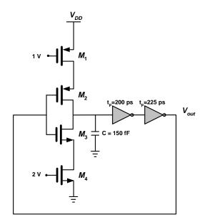
Fig. 6. A three-stage ring oscillator.
