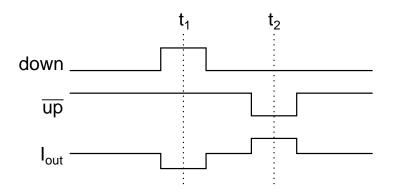
Fig. 2. Timing diagram for the charge pump.
