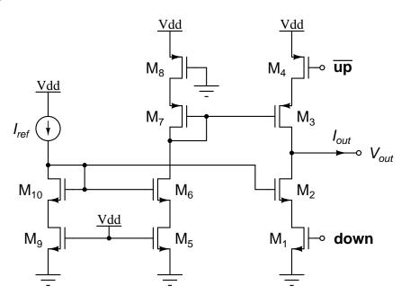
Fig. 1. Charge pump circuit.
