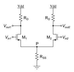
Fig. 3. Differential amplifier circuit biased with non-ideal current source.
