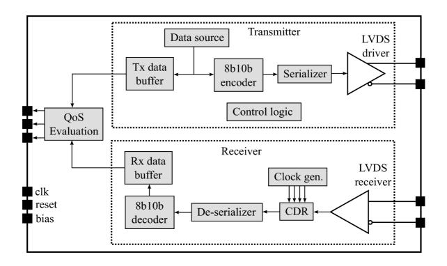
Figure 1: High speed serial link transceiver system overview.
