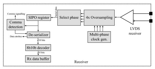
Figure 2: Detailed receiver architecture.
