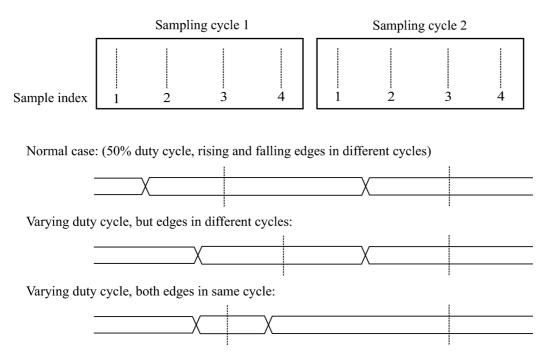
Figure 3: Oversampling data recovery by cycle-to-cycle selection of optimal sampling phase, which adapts to dynamic variations in skew and duty cycle.
