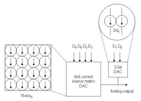
Figure 1. 6-bit DAC divided in 4x4 matrix DAC and a 2-bit DAC
