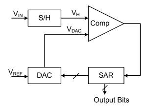
Figure 1: Block diagram of SA ADC
