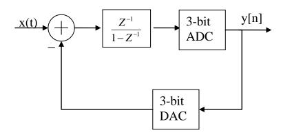
Figure 1: First-order Sigma-Delta modulator architecture.
