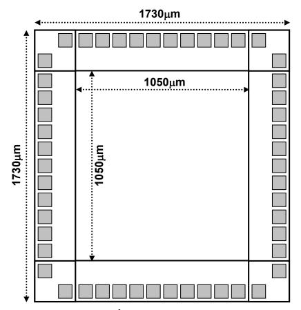
Figure 2: Schematic picture of a  $3\text{mm}^2$  chip with 40 generic pads four  $V_{DD}$  and four  $V_{SS}$  pads (total 48 pads), which will be shared between a number of projects.
