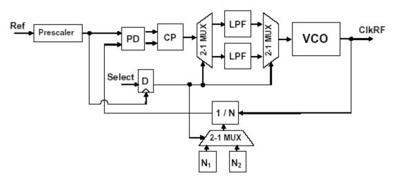
Figure 1: System Block diagram of PLL-based BFSK Modulator
