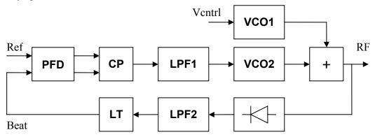
Figure 1: System Block diagram of Beat Frequency Oscillator
